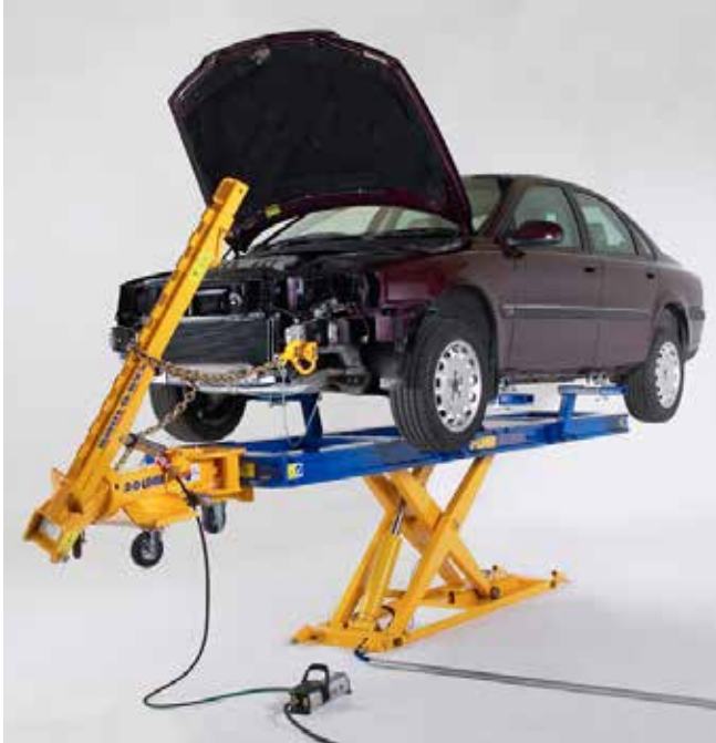
Maximum work space between bench and underside of vehicle with longer bench arms
