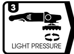
Keep the polishing machine continuously moving and apply light pressure
