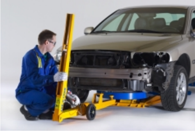
2. It only takes a couple of seconds to “snap-on” SPEED’s convenient 5-ton draw aligner.
