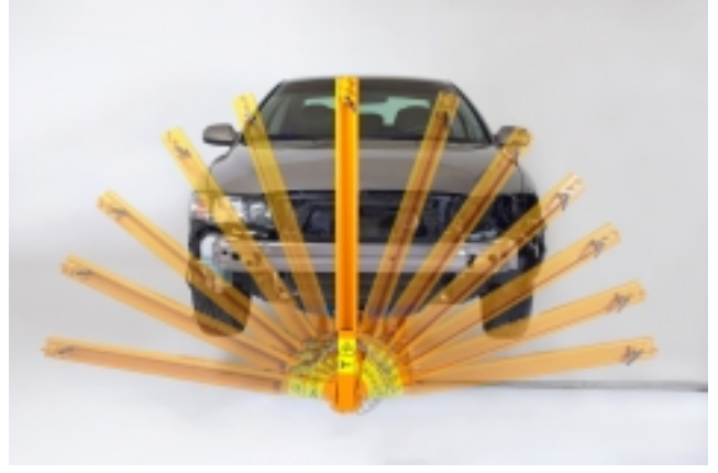
3. The draw aligner can be adjusted to any position. It is self-locking and easy to mount in the right spot.
