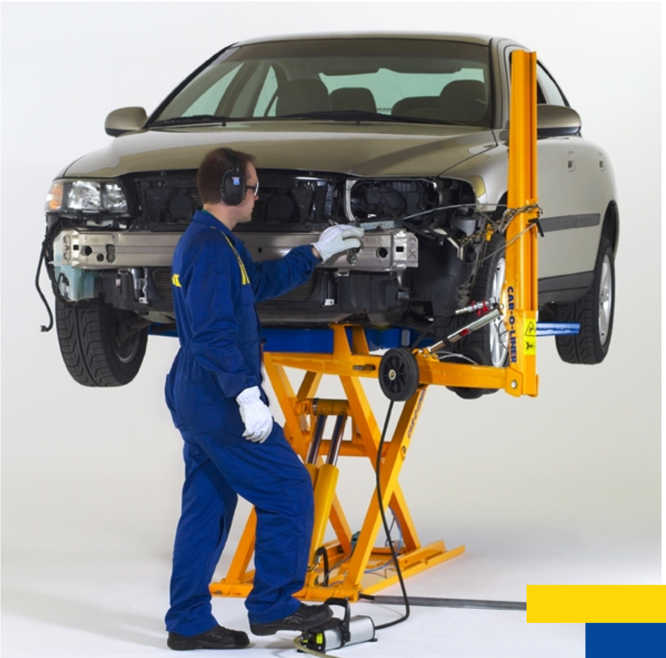
5. Then it’s time to lock the car in position with the chassis clamps and start the aligning work.
