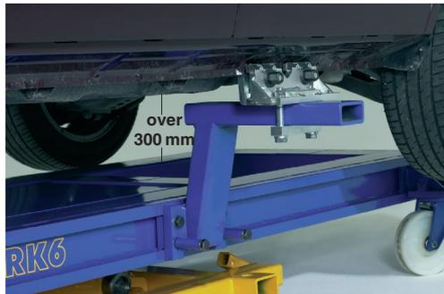
Longer bench arms allow maximum work space between bench and underside of vehicle.
