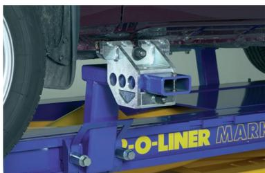
Optional chassis clamp (B110) offers faster setup and removal using just two bolts.
