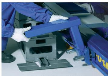
Optional mounting arm (B310) clicks in and out for faster loading and unloading.
