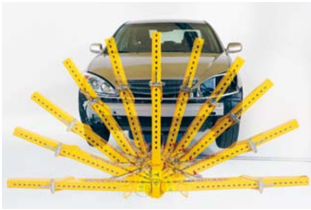
The draw aligner can be adjusted to any position. It is self locking and easy to mount
