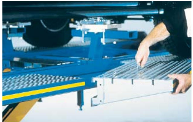
Removable ramp sections lift out easily to give better access to the vehicle.
