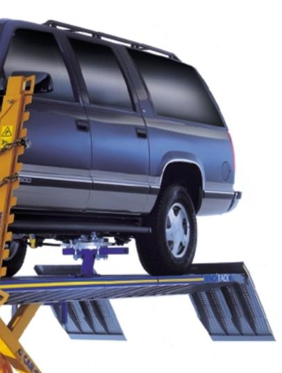
Side support system locks parts in place when pulling, or holds them in place during welding operations.
